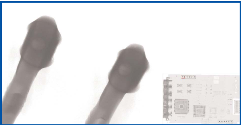
FIGURE 10: X-ray image of two pins in one of the IDC six-pin connectors on an immersion gold finish board that had undergone convection reflow. The pin location is shown by the small highlighted rectangle on the navigation map.
