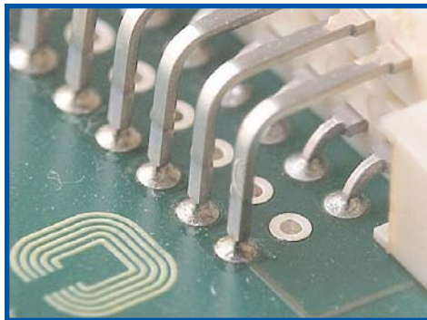
FIGURE 4: Typical topside joints produced using PIHR.
