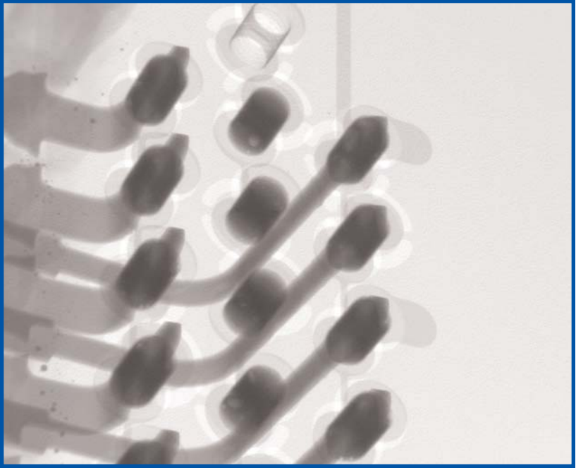
FIGURE 12: Part of 96-pin connector on an OSP board after convection reflow, center contact row not fitted.
