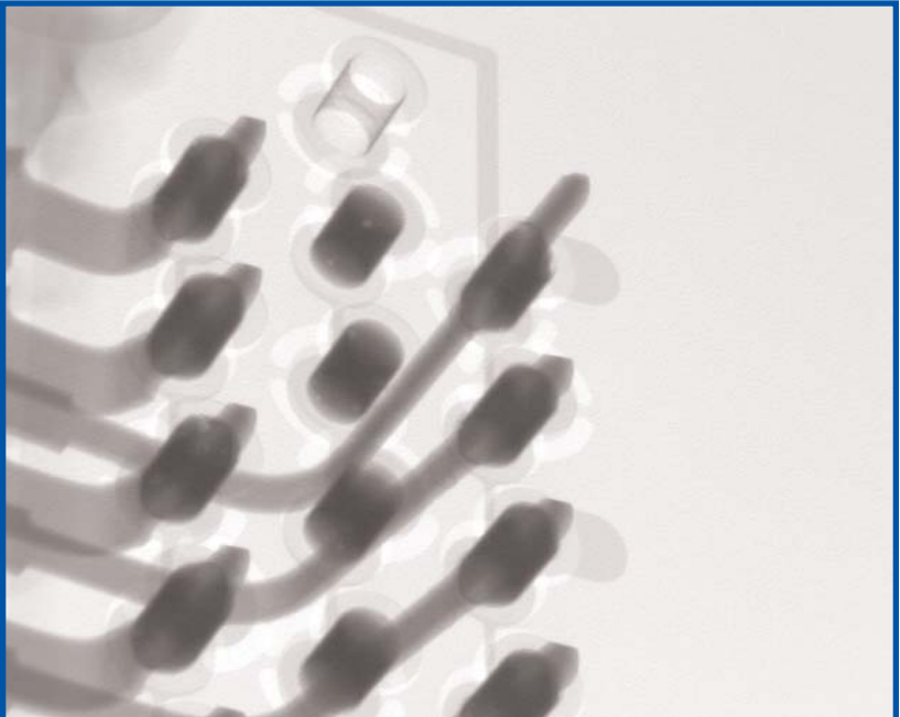
FIGURE 13: Part of 96-pin connector on an ImAg board after convection reflow, center contact row not fitted.
