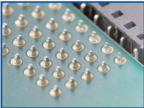
FIGURE 3: Typical bottomside joints produced using PIHR.
