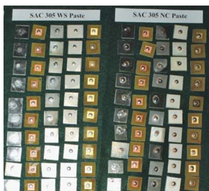
Figure 7. Wetting characteristics of SAC305 water-soluble and no-clean pastes.
