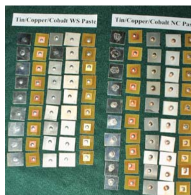
Figure 8. Wetting characteristics of SnCuCo were similar to those of SAC305.
