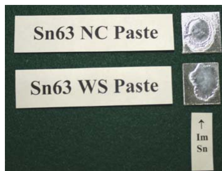
Figure 6. Pastes diffused through immersion tin.
