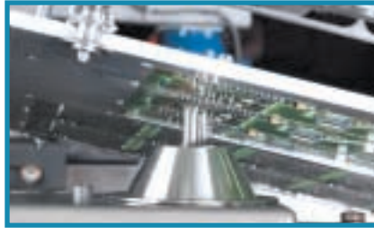
FIGURE 2: Drag soldering with a single nozzle beneath the PCB.
