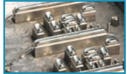
FIGURE 3: Dip soldering using custom nozzle plate.
