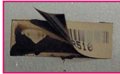
FIGURE 3: Polyimide label subjected to 300°C for 50 minutes.
