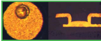
FIGURE 1: (left) Top view of 0.015 in. pad with 0.005 in. via and (right) side view of 0.011 in. pad with 0.005 in. via.
