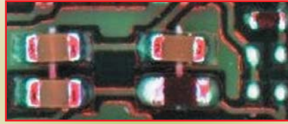
FIGURE 2: AOI systems can identify excess solder conditions that can occur in smaller pads, which are typical in lead-free designs.
