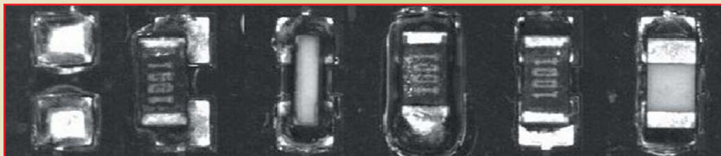
FIGURE 1: Examples of 0603 defects on a lead-free PCB.
