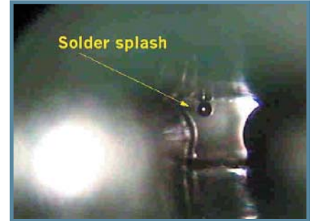
FIGURE 5: Tiny solder balls.
