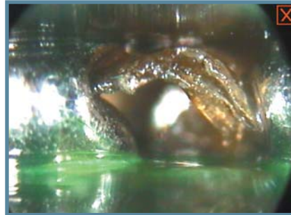
FIGURE 4: Flux residue under package.
