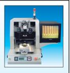
trolled equipment that produces uniform and precise temperature distribution, fast heating and cool-down. The Pulse Heat Bonder and Soldering Systems offer a wide range of programmable profiles for targeted idle (to 150°C), with preheat and reflow temperatures (to 500°C). The many applications include edge connectors to PCB, TAB to PCB, Hot Bar Reflow, Soldering and other uses. Optional B&W camera system. Rotary 2-station also available. From \$10,500.
