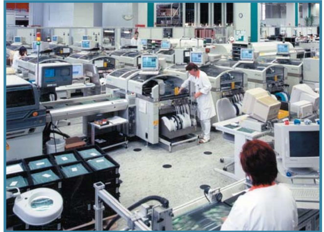
FIGURE 2: Common and modular machine elements, such as feeders and programming, make workcells product-oriented and permit staff to control activity at the cell level.
