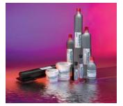
SynTech-LF lead-free, no-clean solder paste is made with synthetic poly adduct components. Compatible with SnAg and SnAgCu alloys. Leaves nonconductive, noncorrosive, post-reflow residue as a protective coating. Said to have 12-hr. stencil life and 12-16 hr. tack time, and requires no refrigeration. ICT friendly, compatible with OSPs.
