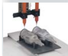
APPLYING SEAL MOTOR HOUSINGS
