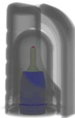
Figure 3: Slice through a Rotring (courtesy Procon X-Ray).
