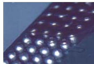
Figure 6: Inadequate vertical fill.
