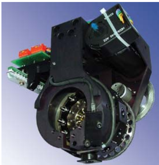
The 12-position turret head, called Tornado, uses the 3DPS adaptive positioning software and contact sensor system.
