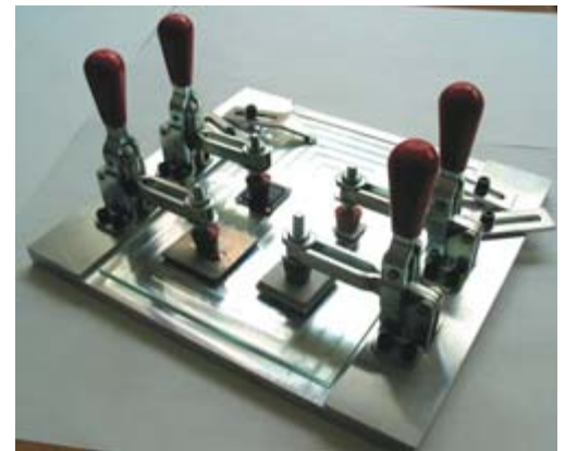
Figure 1: Underfill fixture, with typical glass slide.
