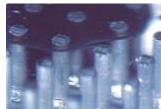
Figure 8: Columns exhibit too-low viscosity.
