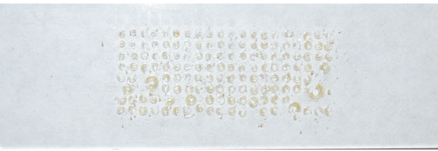
(c) Flux residue after removal of solder ball
